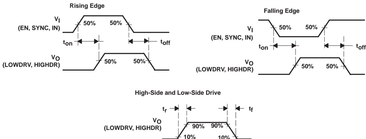
Figure 1. Voltage Waveforms
