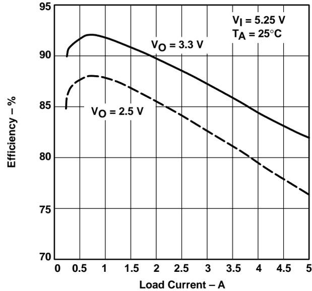
Figure 26. Converter Efficiency
