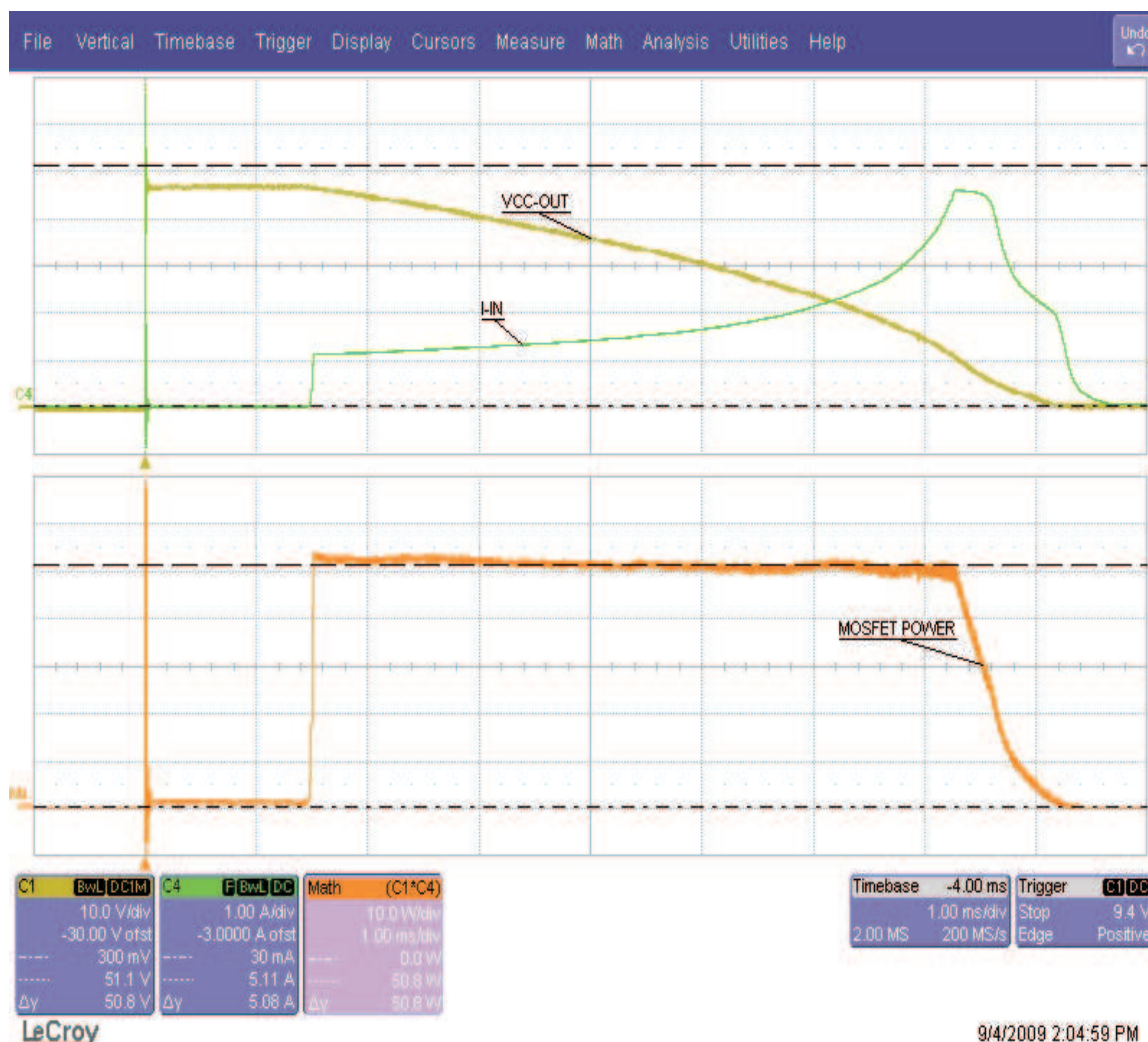
Figure 13. Computation of the External FET Stress During Startup
