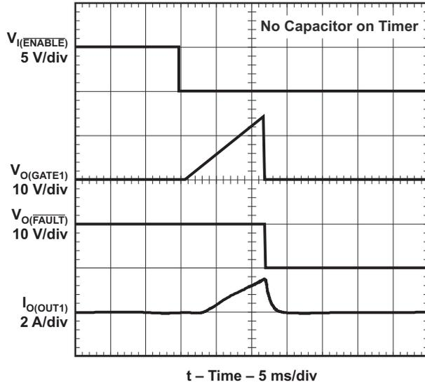
**Figure 5. Channel 1 Overcurrent Response: Enabled Into Overcurrent Load**
