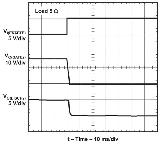
Figure 4. Turnoff Voltage Transition of Channel 2
