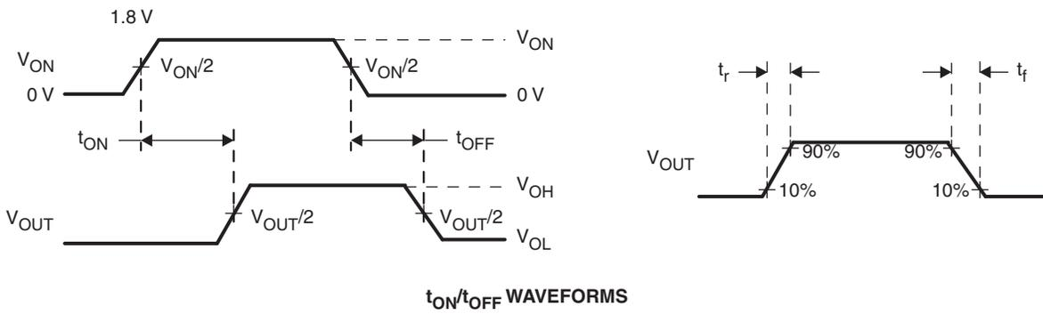
A.  $t_{rise}$  and  $t_{fall}$  of the control signal is 100 ns.
