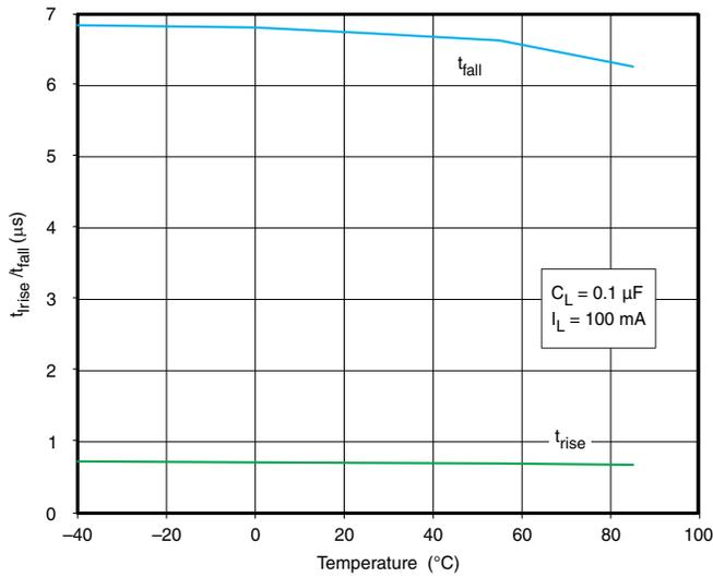
Figure 12.  $t_{rise}$  (TPS22903/4) /  $t_{fall}$  (TPS22903) vs Temperature ( $V_{IN} = 3.3\text{ V}$ )
