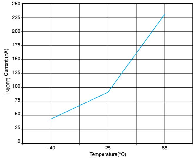
Figure 8.  $I_{IN(OFF)}$  vs Temperature ( $V_{IN} = 3.3$  V)
