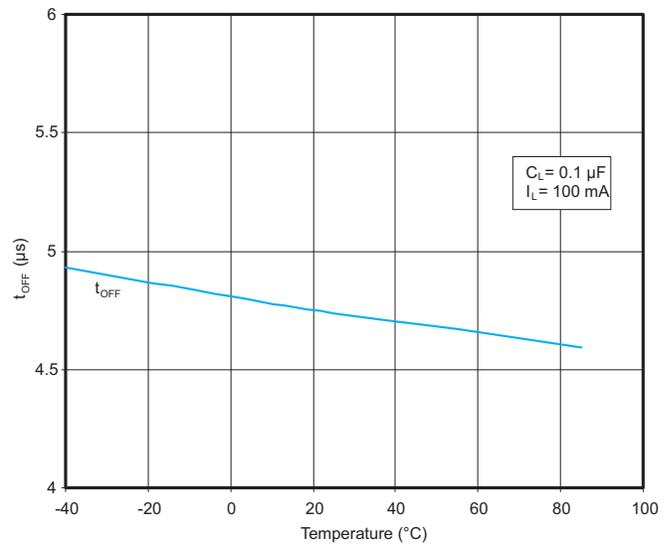
Figure 15.  $t_{OFF}$  (TPS22904) vs Temperature ( $V_{IN} = 3.3\text{ V}$ )
