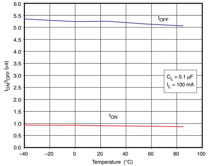
Figure 13.  $t_{ON}$  (TPS22903/4) /  $t_{OFF}$  (TPS22903) vs Temperature ( $V_{IN} = 3.3\text{ V}$ )
