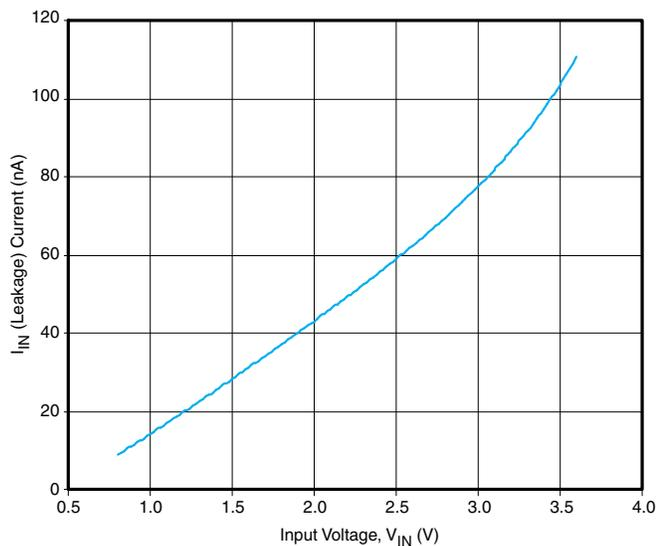
Figure 9.  $I_{IN}(\text{Leakage})$  vs  $V_{IN}$  ( $I_{OUT} = 0$ )
