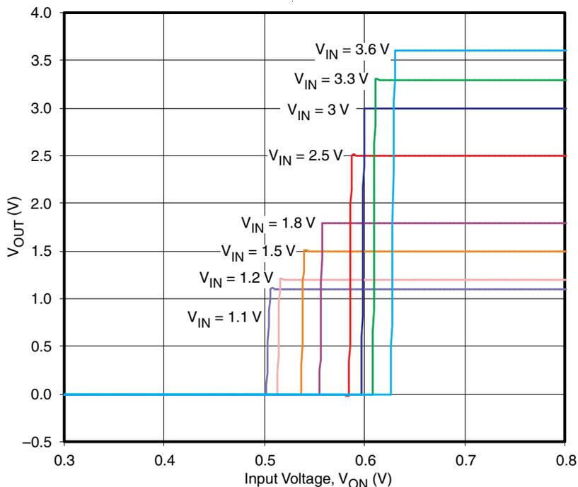
Figure 11. ON-Input Threshold
