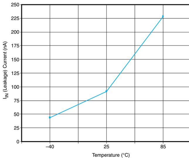
Figure 10.  $I_{IN}(\text{Leakage})$  vs Temperature ( $V_{IN} = 3.3$  V)
