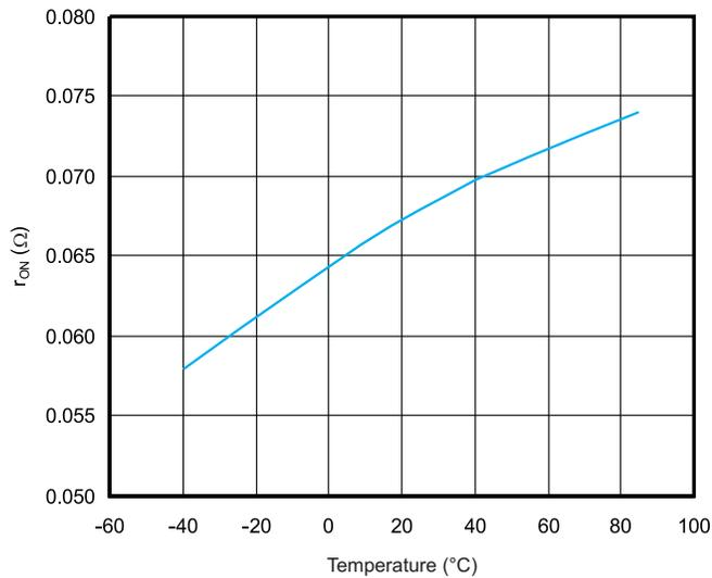
Figure 3.  $r_{ON}$  vs Temperature ( $V_{IN} = 3.3$  V)
