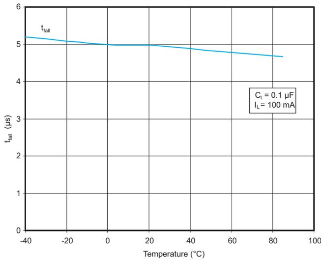
Figure 14.  $t_{fall}$  (TPS22904) vs Temperature ( $V_{IN} = 3.3\text{ V}$ )
