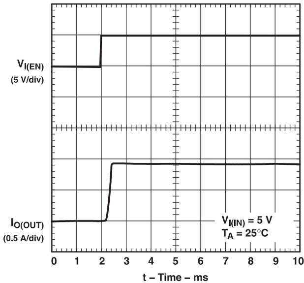
Figure 6. TPS2080, Short-Circuit Current, Device Enabled Into Short
