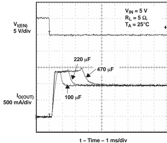
Figure 7. Inrush Current With Different Load Capacitance
