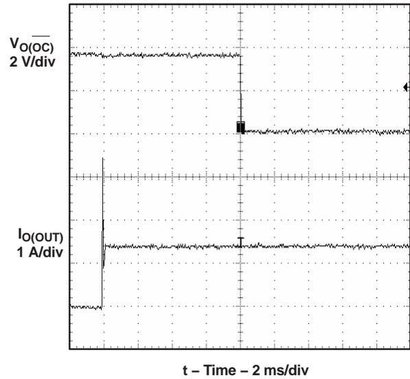
Figure 9. 1- $\Omega$  Load Connected to Enabled Device
