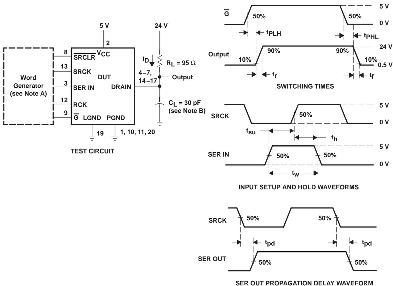
Figure 2. Test Circuit, Switching Times, and Voltage Waveforms
