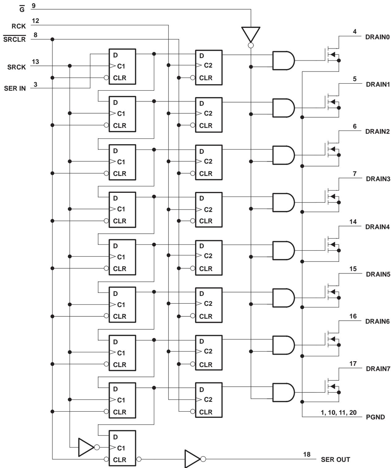
**schematic of inputs and outputs**
