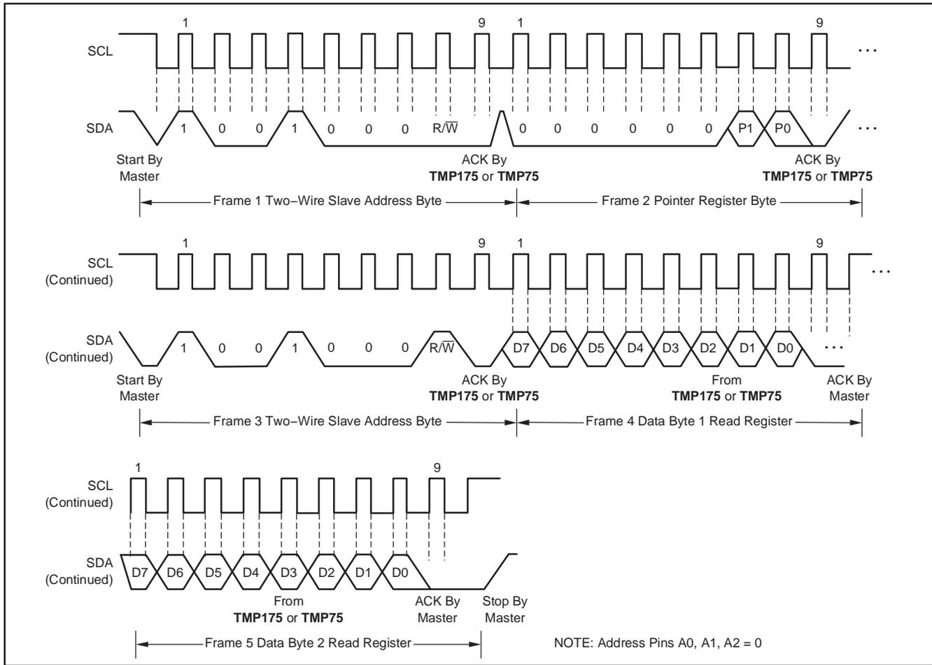
**Figure 7. Two-Wire Timing Diagram for Read Word Format**
