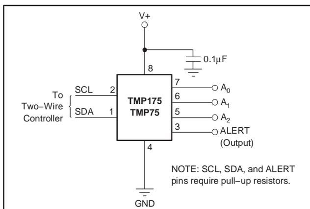
Figure 1. Typical Connections of the TMP175 and TMP75
