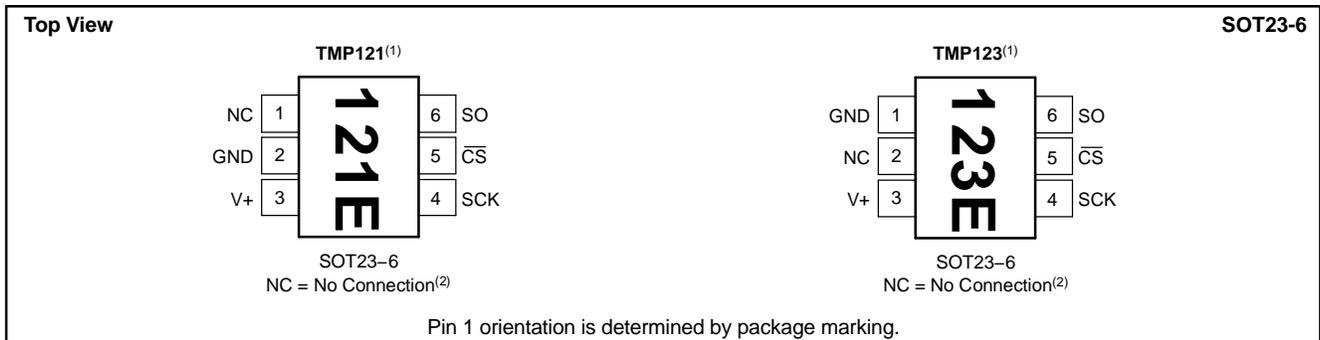
(1) Pin 1 of the SOT23-6 package is determined by orienting the package marking as shown.
