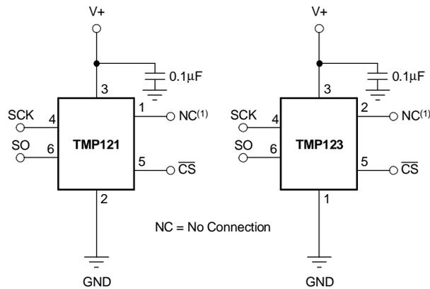
NOTE: Pins labeled NC should be left floating or connected to GND.
