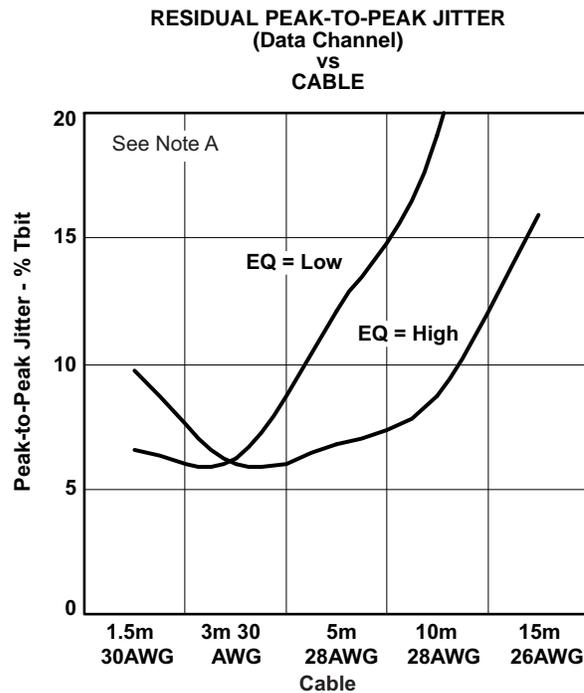
A. 1080p 12-Bit,  $V_{CC} = AV_{CC} = 3.3\text{ V}$ ,  $T_A = 25^\circ\text{C}$ ,  $R_{VSADJ} = 4.02\text{ k}\Omega$ , See [Figure 6](#), Clock Channel = 222.8 MHz, Data Channel = 2.228 Gbps
