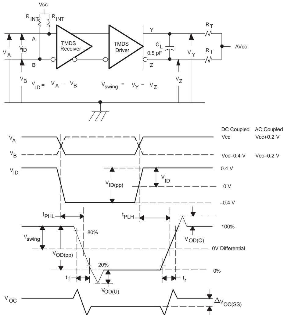
NOTE: All input pulses are supplied by a generator having the following characteristics:  $t_r$  or  $t_f < 100\text{ ps}$ , 100 MHz from Agilent 81250.  $C_L$  includes instrumentation and fixture capacitance within 0.06 m of the D.U.T. Measurement equipment provides a bandwidth of 20 GHz minimum.
