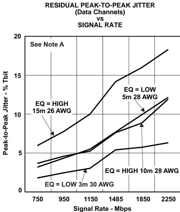
A. Channels 2, 3, 4,  $V_{CC} = AV_{CC} = 3.3\text{ V}$ ,  $T_A = 25^\circ\text{C}$ ,  $R_{VSADJ} = 4.02\text{ k}\Omega$ , See Figure 6
