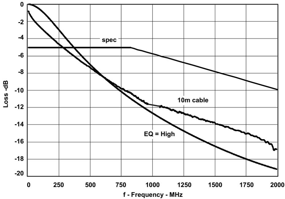
Figure 15. Frequency Response Compensation Curve at EQ = H
