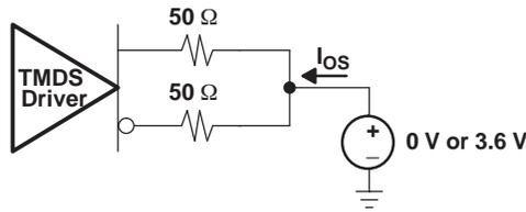
Figure 3. Short Circuit Output Current Test Circuit
