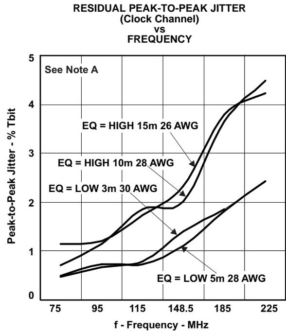
A. Channel 1,  $V_{CC} = AV_{CC} = 3.3\text{ V}$ ,  $T_A = 25^\circ\text{C}$ ,  $R_{VSADJ} = 4.02\text{ k}\Omega$ , See Figure 6
