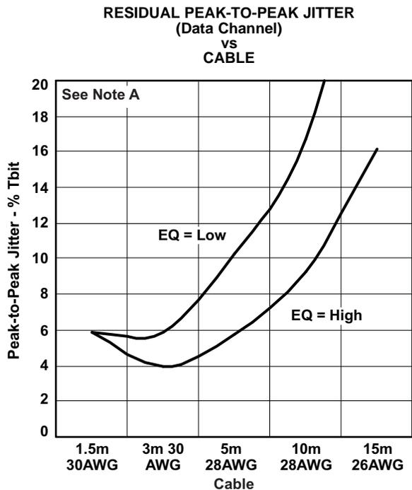
A. 1080p 10-Bit,  $V_{CC} = AV_{CC} = 3.3\text{ V}$ ,  $T_A = 25^\circ\text{C}$ ,  $R_{VSADJ} = 4.02\text{ k}\Omega$ , See [Figure 6](#), Clock Channel = 185.6 MHz, Data Channel = 1.856 Gbps
