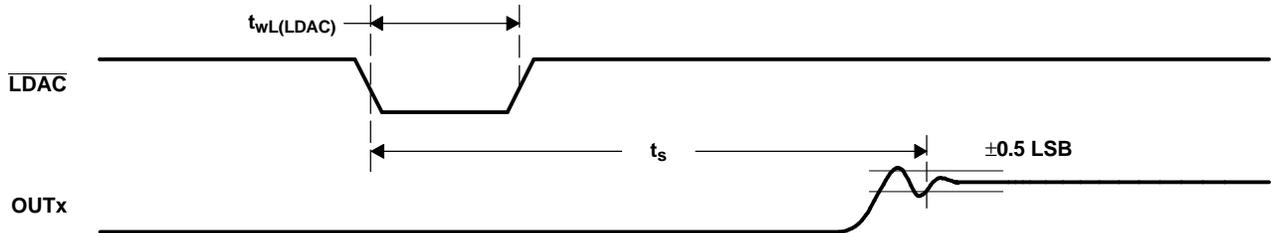
Figure 2. Output Timing
