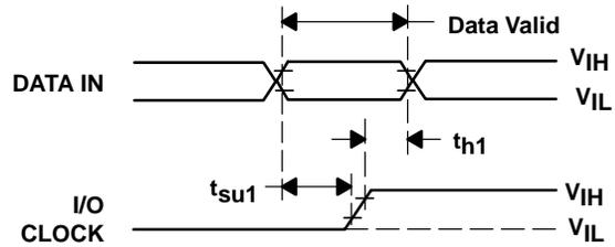
Figure 26. DATA IN and I/O CLOCK Voltage
