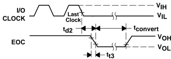
Figure 29. I/O CLOCK and EOC Voltage Waveforms
