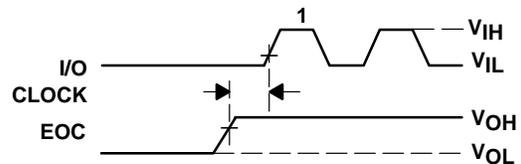
Figure 32. I/O CLOCK and DATA OUT Voltage
