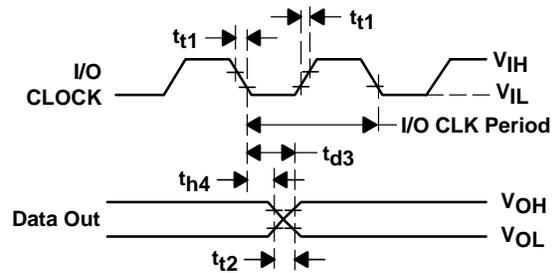
Figure 28. I/O CLOCK and DATA OUT Voltage Waveforms
