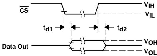
Figure 25. DATA OUT to Hi-Z Voltage Waveforms
