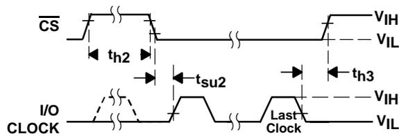
Figure 27.  $\overline{\text{CS}}$  and I/O CLOCK Voltage Waveforms
