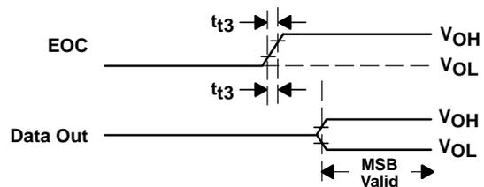
Figure 30. EOC and DATA OUT Voltage Waveforms
