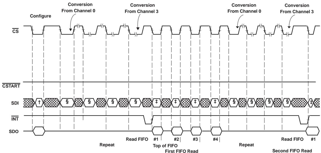
† Command = Configure write for mode 10 or 11, FIFO threshold = 1/2, sweep seq = 0–1–2–3.
