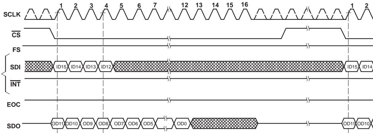
These devices can perform continuous FIFO read cycles (FS = 1) controlled by SCLK; SCLK can stop between each 16 SCLKs.
