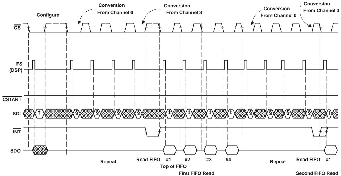
† Command = Configure write for mode 10 or 11, FIFO threshold = 1/2, sweep seq = 0–1–2–3.
