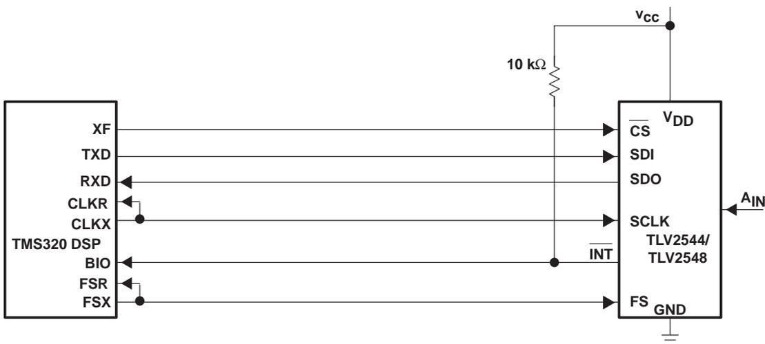
Figure 38. Typical Interface to a TMS320 DSP™
