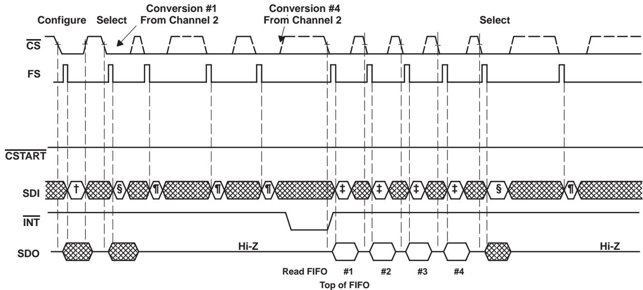
† Command = Configure write for mode 01, FIFO threshold = 1/2
