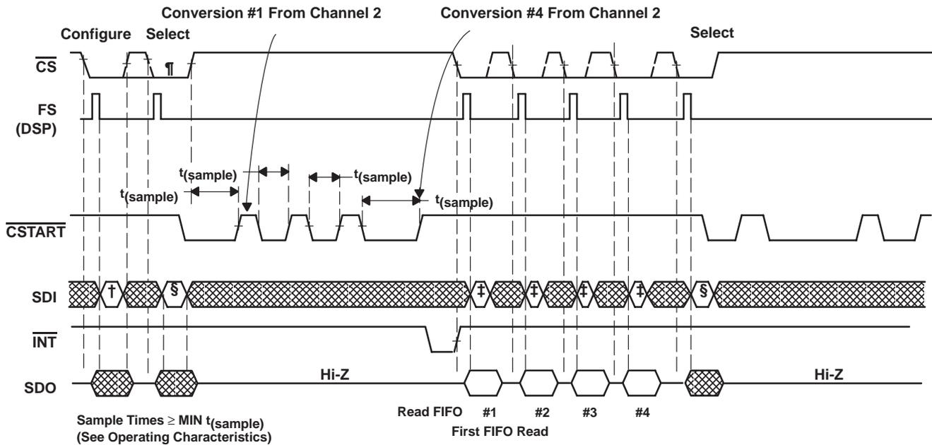
† Command = Configure write for mode 01, FIFO threshold = 1/2
