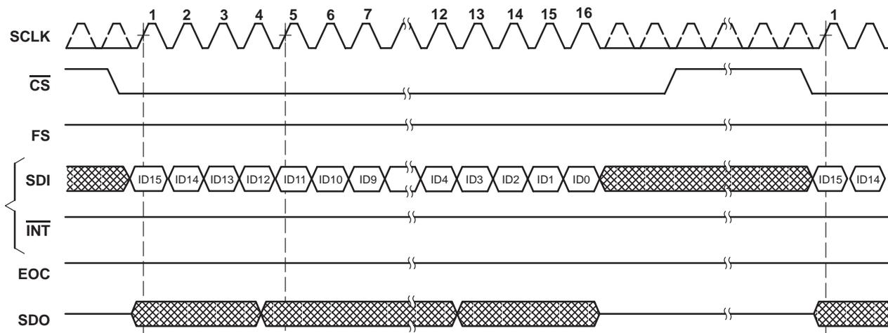
**Figure 6. TLV2544/TLV2548 Write Cycle (FS = 1)**
