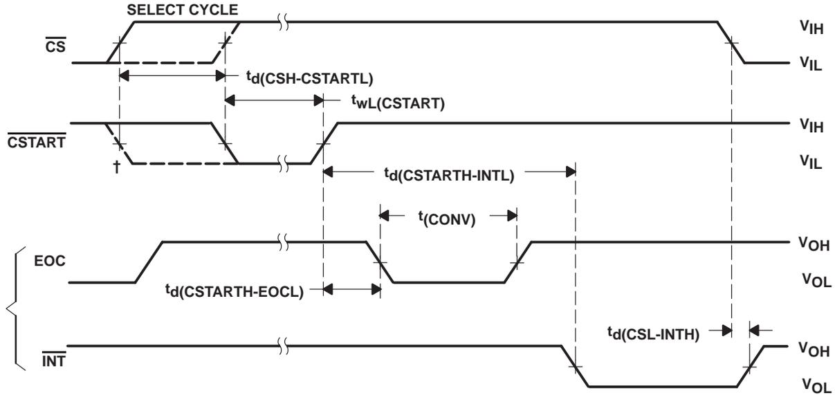
† CSTART falling edge may come before the rising edge of CS but no sooner than the fifth SCLK of the SELECT CYCLE.
