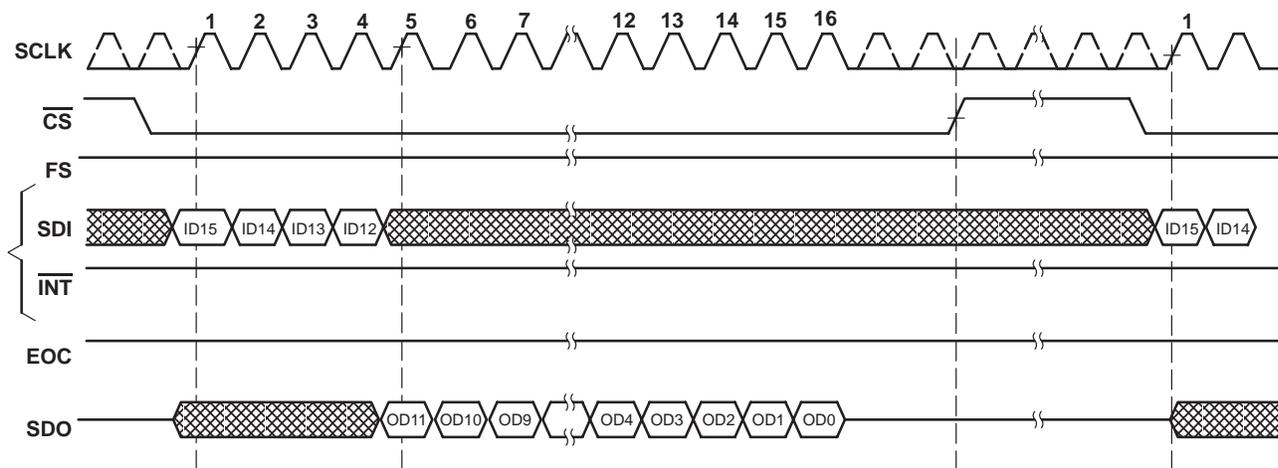
**Figure 3. TLV2544/TLV2548 Read CFR Cycle (FS = 1)**
