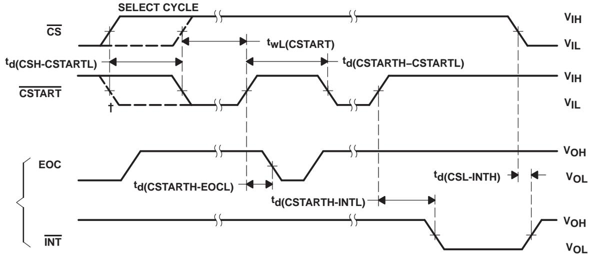
† CSTART falling edge may come before the rising edge of CS but no sooner than the fifth SCLK of the SELECT CYCLE. In this case, the actual sampling time is measured from the rising edge of CS to the rising edge of CSTART.
