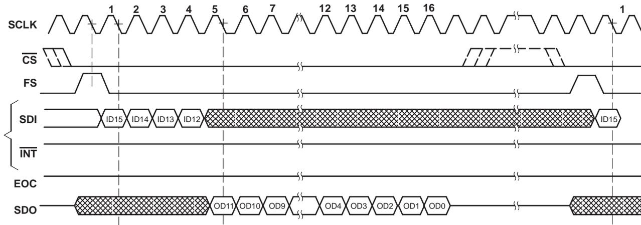
**Figure 2. TLV2544/TLV2548 Read CFR Cycle (FS active)**
