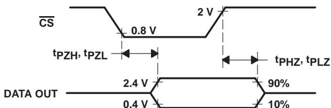
Figure 3. DATA OUT to Hi-Z Voltage Waveforms
