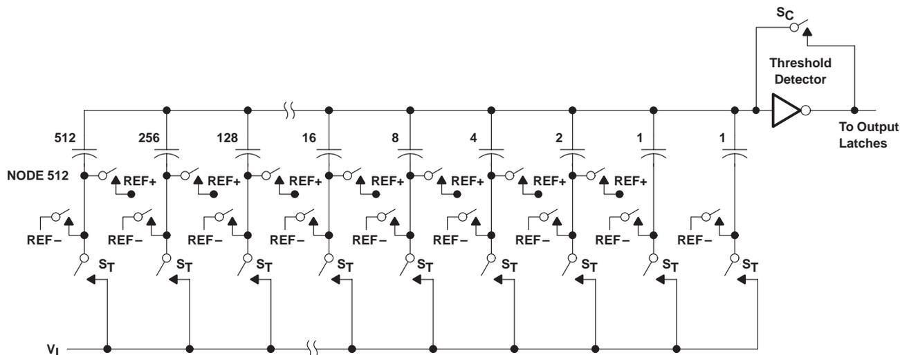
Figure 1. Simplified Model of the Successive-Approximation System
