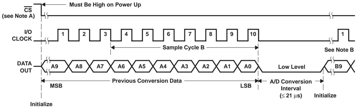
Figure 7. Timing for 10-Clock Transfer Not Using  $\overline{CS}$
