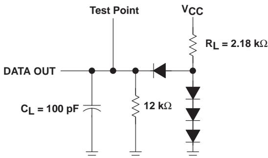
Figure 2. Load Circuit
