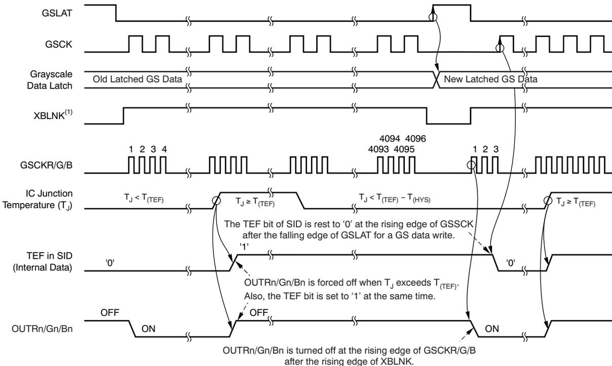
(1) The following internal signal also works to turn the constant outputs on as same as XBLNK inputting. The internal blank signal is generated when GSLAT is input for GS data with display timing reset enabled. Also, the signal is generated at the 4096th GSCKR/G/B when auto repeat mode is enabled. XBLNK can be connected to VCC when the display timing reset or auto repeat is enabled.
