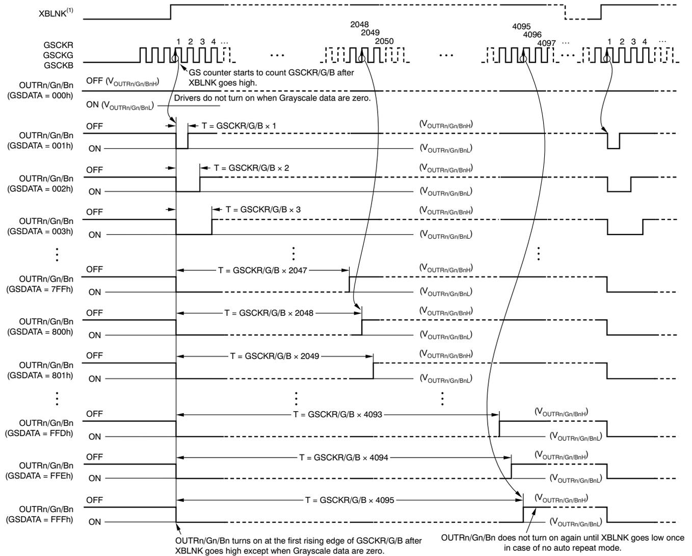
(1) The internal blank signal is generated when GSLAT is input for GS data with display timing reset enabled. Also, the signal is generated at 4096th GSKCR/G/B when the auto repeat mode is enabled. XBLNK can be connected to VCC when the display timing reset or auto repeat is enabled.
