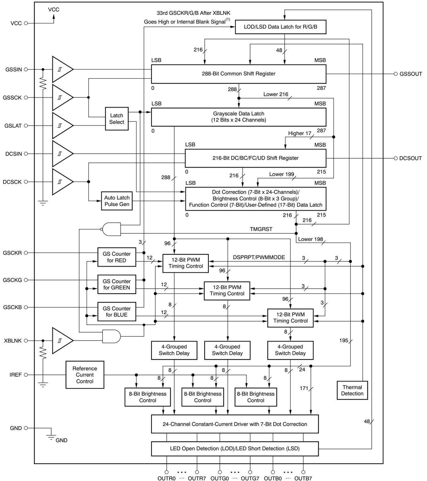
(1) The internal blank signal is generated when GSLAT is input for GS data with display timing reset enabling. Furthermore, the signal is generated at the 4096th GSK when auto repeat mode is enabled. XBLNK can be connected to V<sub>CC</sub> when the display timing reset or auto repeat is enabled.
