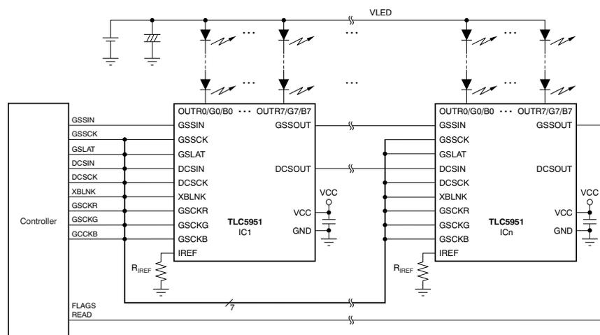
Typical Application Circuit (Multiple Daisy-Chained TLC5951s)
