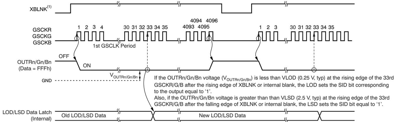
(1) The internal blank signal is generated when GSLAT is input for GS data with display timing reset enabled. Also, the signal is generated at the 4096th GSCK when auto repeat mode is enabled. XBLNK can be connected to VCC when the display timing reset or auto repeat is enabled.
