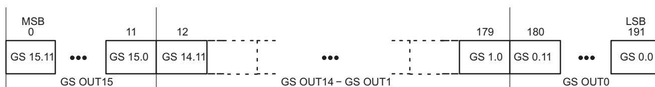
Figure 17. Grayscale Data Packet Format
