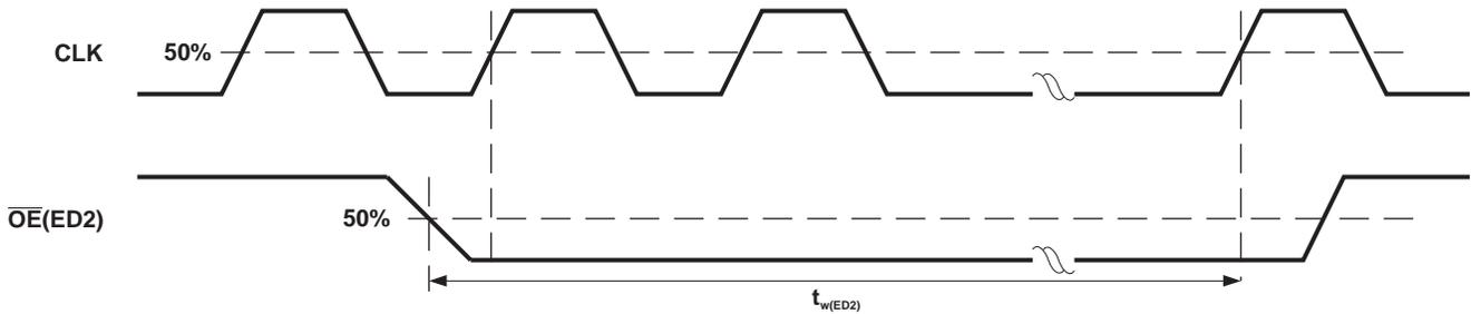
Figure 10. Reading Error Status Code Timing Waveforms
