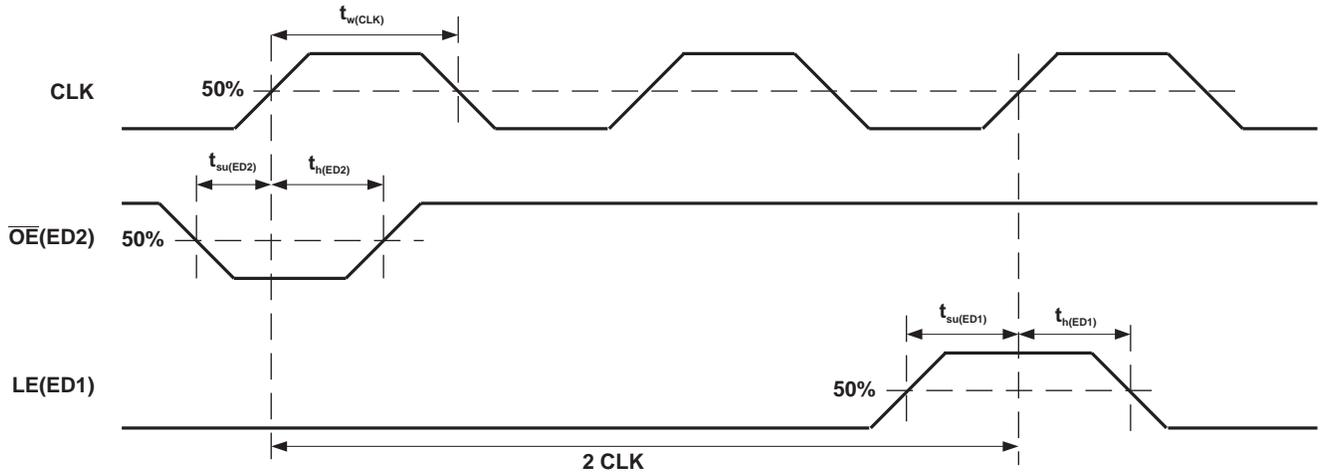
Figure 9. Switching to Special Mode Timing Waveforms
