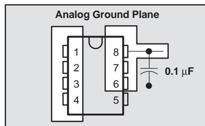
Figure 15. Power-Supply Bypassing
