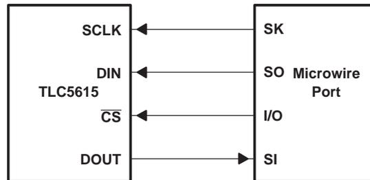
NOTE A: The DOUT-SI connection is not required for writing to the TLC5615 but may be used for verifying data transfer if desired.
