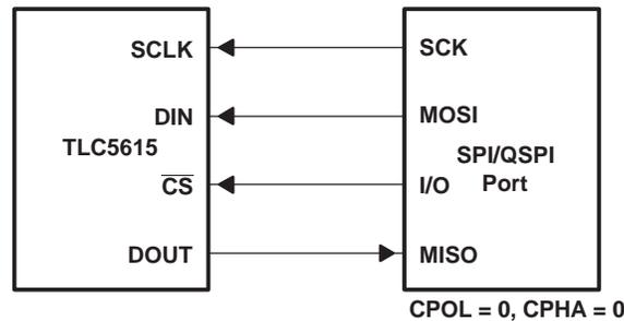
NOTE A: The DOUT-MISO connection is not required for writing to the TLC5615 but may be used for verifying data transfer.
