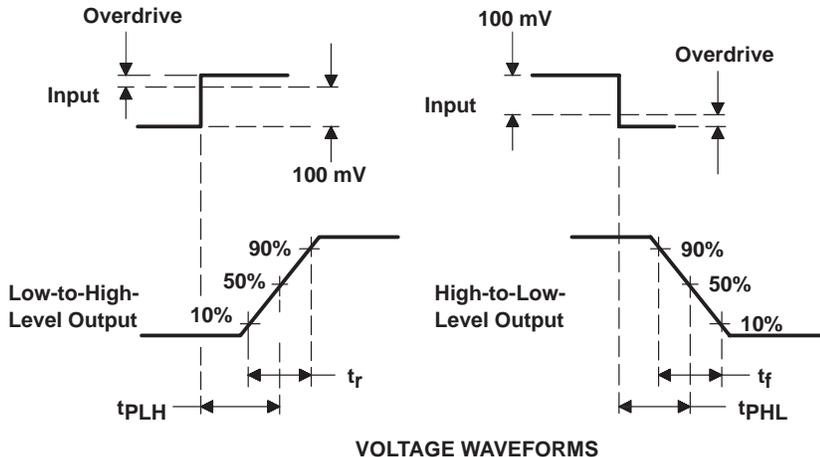
NOTE A:  $C_L$  includes probe and jig capacitance.
