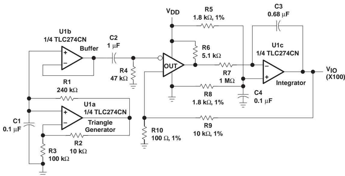
Figure 2. Test Circuit for Input Offset Voltage Measurement
