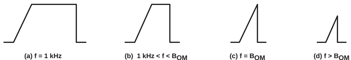
Figure 5. Full-Power-Response Output Signal
