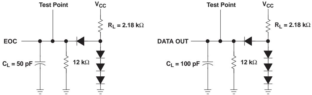
Figure 2. Load Circuits
