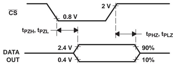
Figure 3. DATA OUT Enable and Disable Voltage Waveforms
