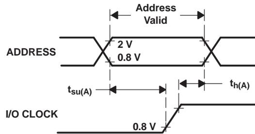
Figure 4. ADDRESS Setup and Hold Time Voltage Waveforms
