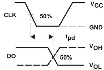
**Figure 2. Data-Output Timing**
