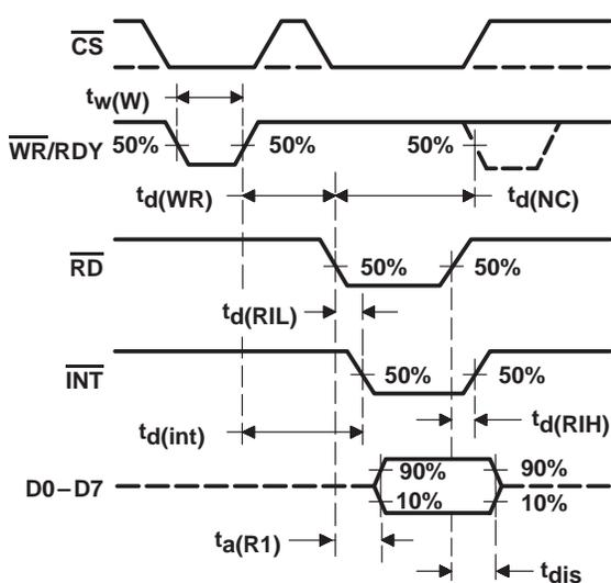
Figure 2. Write-Read-Mode Waveforms
