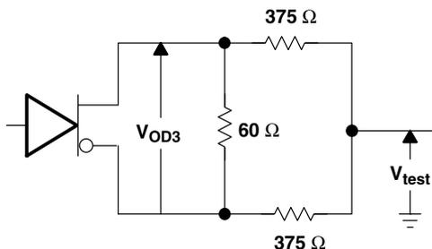
Figure 2. Driver  $V_{OD3}$
