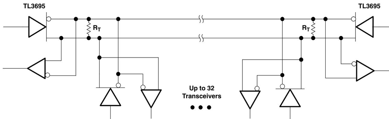
NOTE A: The line should be terminated at both ends in its characteristic impedance ( $R_T = Z_0$ ). Stub lengths off the main line should be kept as short as possible.
