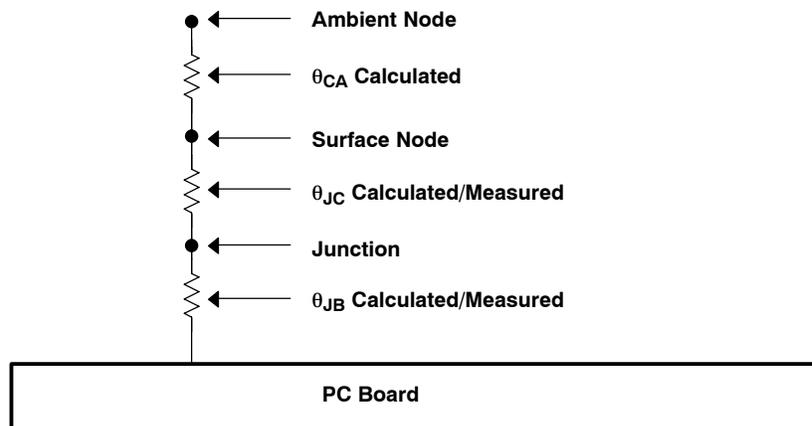
Figure 1. Thermal Resistance
