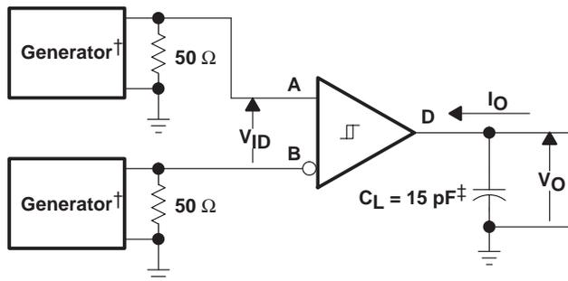
† PRR = 1 MHz, 50% Duty Cycle,  $t_r < 6$  ns,  $t_f < 6$  ns,  $Z_0 = 50 \Omega$
