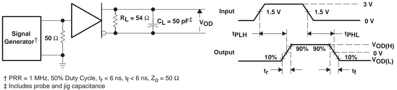
† PRR = 1 MHz, 50% Duty Cycle,  $t_r < 6$  ns,  $t_f < 6$  ns,  $Z_0 = 50 \Omega$
