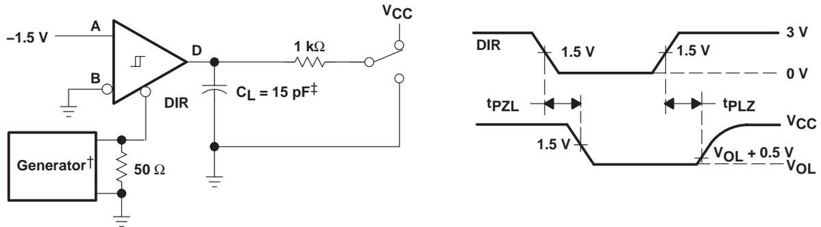
† PRR = 1 MHz, 50% Duty Cycle,  $t_r < 6$  ns,  $t_f < 6$  ns,  $Z_0 = 50 \Omega$
