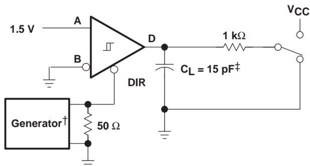
† PRR = 1 MHz, 50% Duty Cycle,  $t_r < 6$  ns,  $t_f < 6$  ns,  $Z_0 = 50 \Omega$
