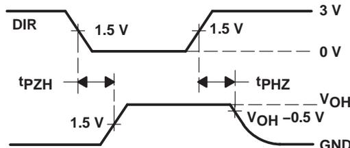
Figure 10. Receiver Enable/Disable Test, High Output
