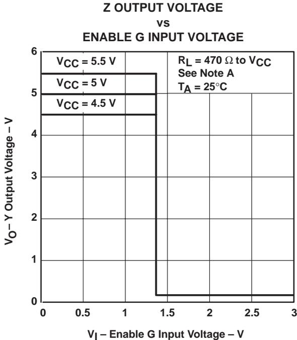
NOTE A: The A input is connected to  $V_{CC}$  during the testing of the Y outputs and to ground during the testing of the Z outputs.
