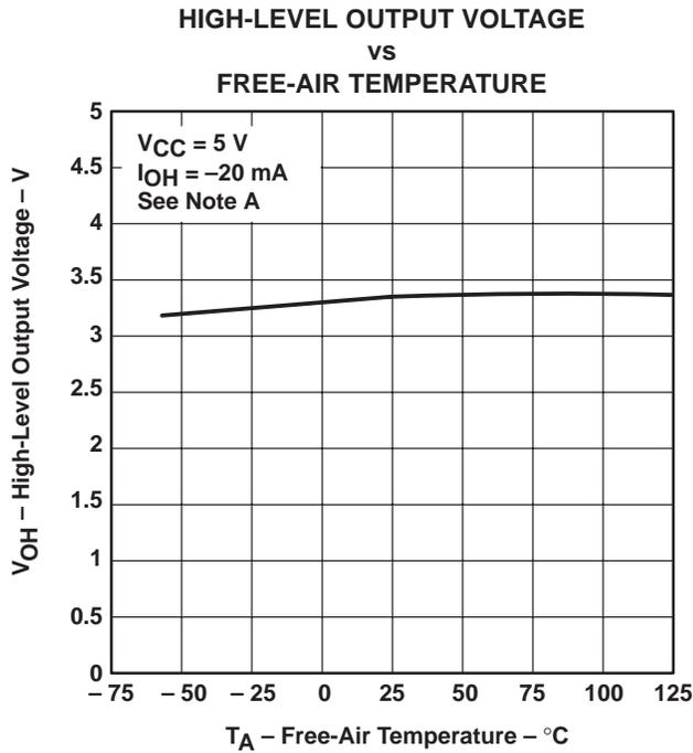
NOTE A: The A input is connected to  $V_{CC}$  during the testing of the Y outputs and to ground during the testing of the Z outputs.
