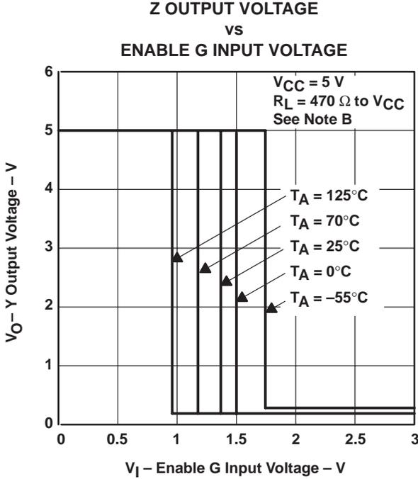
NOTE B: The A input is connected to GND during the testing of the Y outputs and to  $V_{CC}$  during the testing of the Z outputs.
