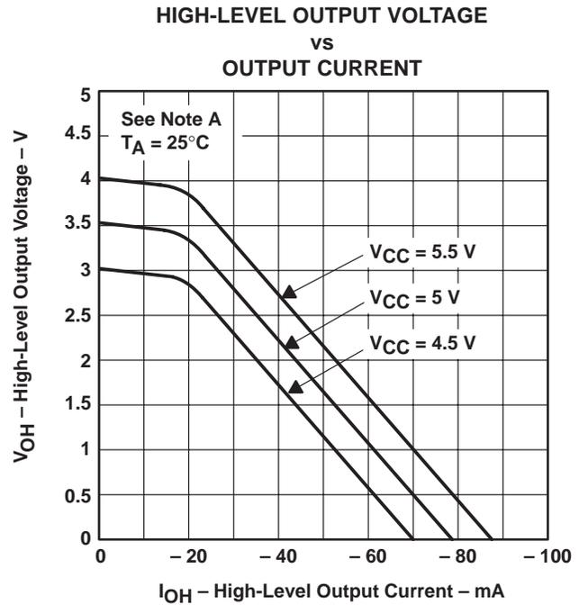
NOTE A: The A input is connected to  $V_{CC}$  during the testing of the Y outputs and to ground during the testing of the Z outputs.
