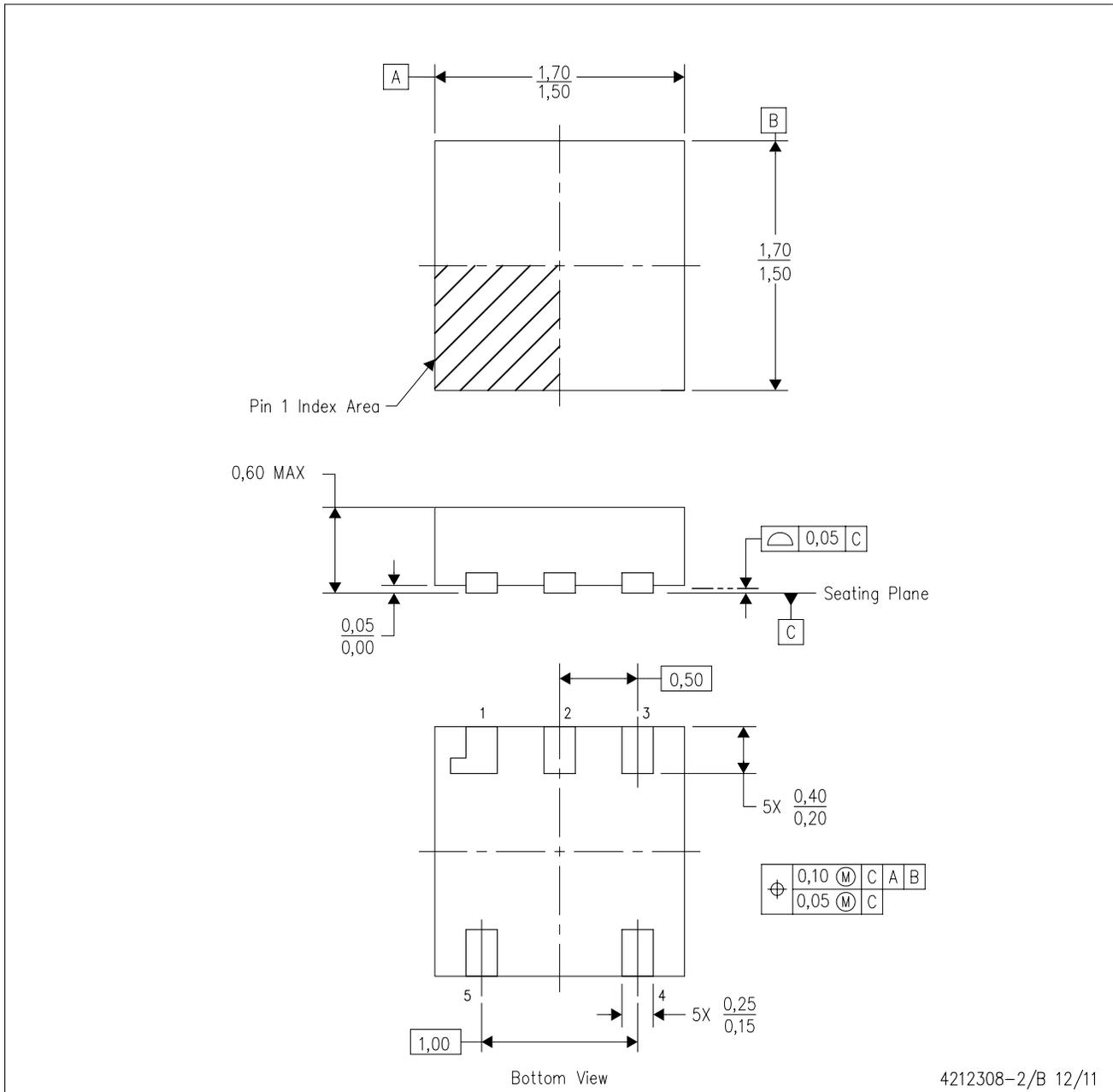
NOTES: A. All linear dimensions are in millimeters. Dimensioning and tolerancing per ASME Y14.5M-1994.
