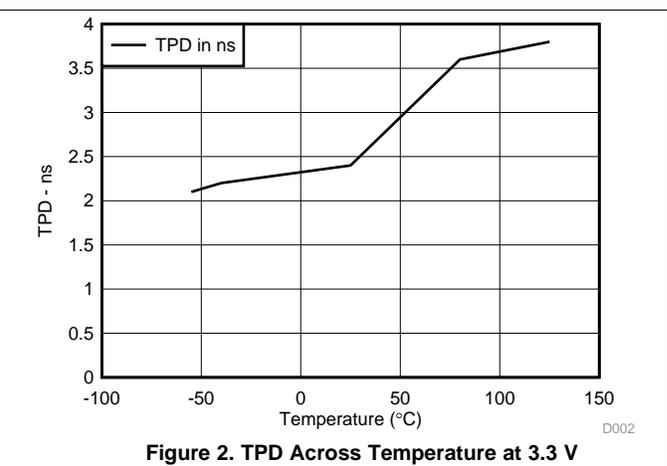
Figure 2. TPD Across Temperature at 3.3V
