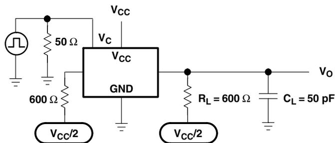
Figure 8. Crosstalk (Control Input – Switch Output)
