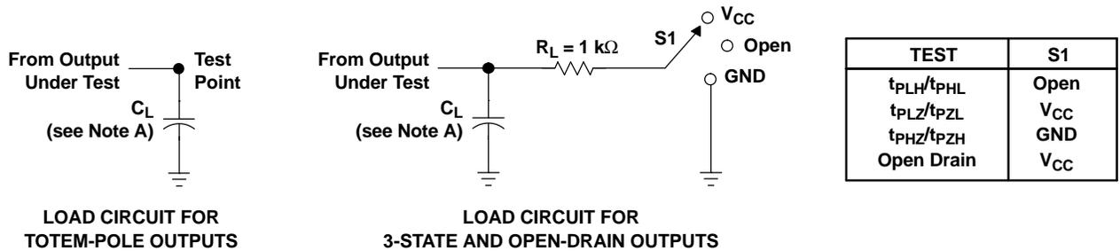
LOAD CIRCUIT FOR TOTEM-POLE OUTPUTS
