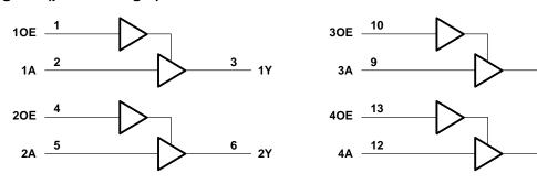
Pin numbers shown are for the D, DB, DGV, J, NS, PW, and W packages.
