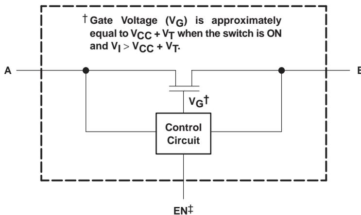
‡ EN is the internal enable signal applied to the switch.
