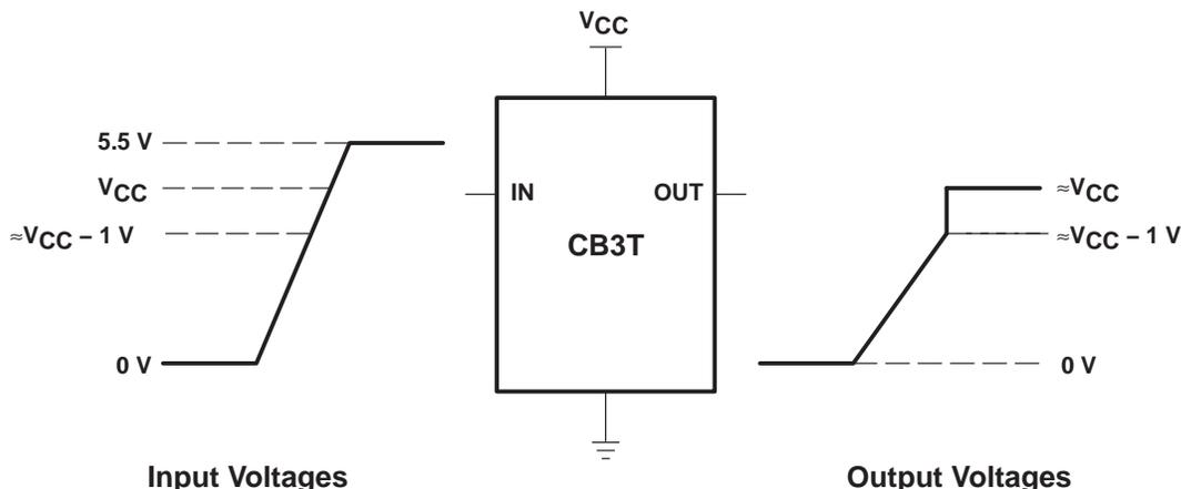
NOTE A: If the input high voltage ( $V_{IH}$ ) level is greater than or equal to  $V_{CC} - 1\text{ V}$ , and less than or equal to 5.5 V, the output high voltage ( $V_{OH}$ ) level will be equal to approximately the  $V_{CC}$  voltage level.
