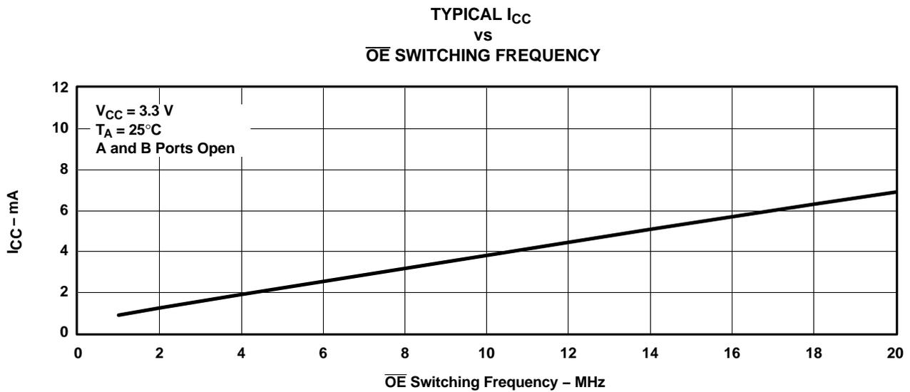
Figure 2. Typical  $I_{CC}$  vs  $\overline{OE}$  Switching Frequency
