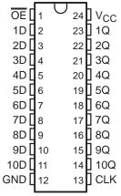
The ten flip-flops are edge-triggered D-type flip-flops. On the positive transition of the clock, the Q outputs will be true to the data (D) inputs.
