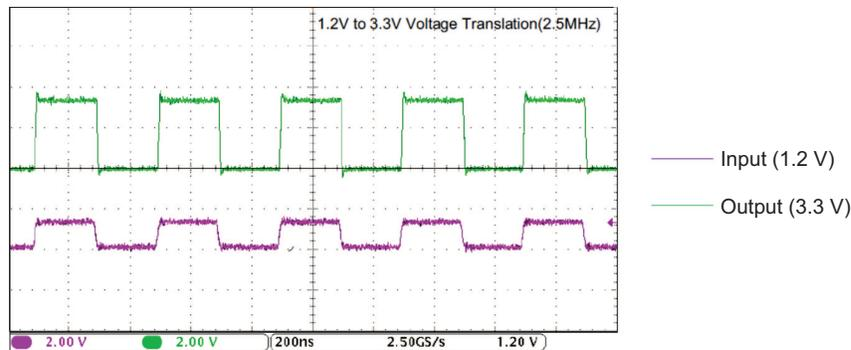
**Figure 13. Translation Up (1.2 V to 3.3 V) at 2.5 MHz**
