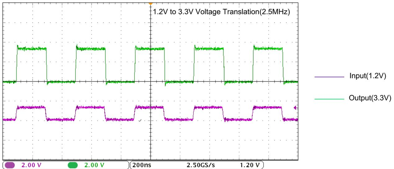
**Figure 12. Translation Up (1.2 V to 3.3 V) at 2.5 MHz**
