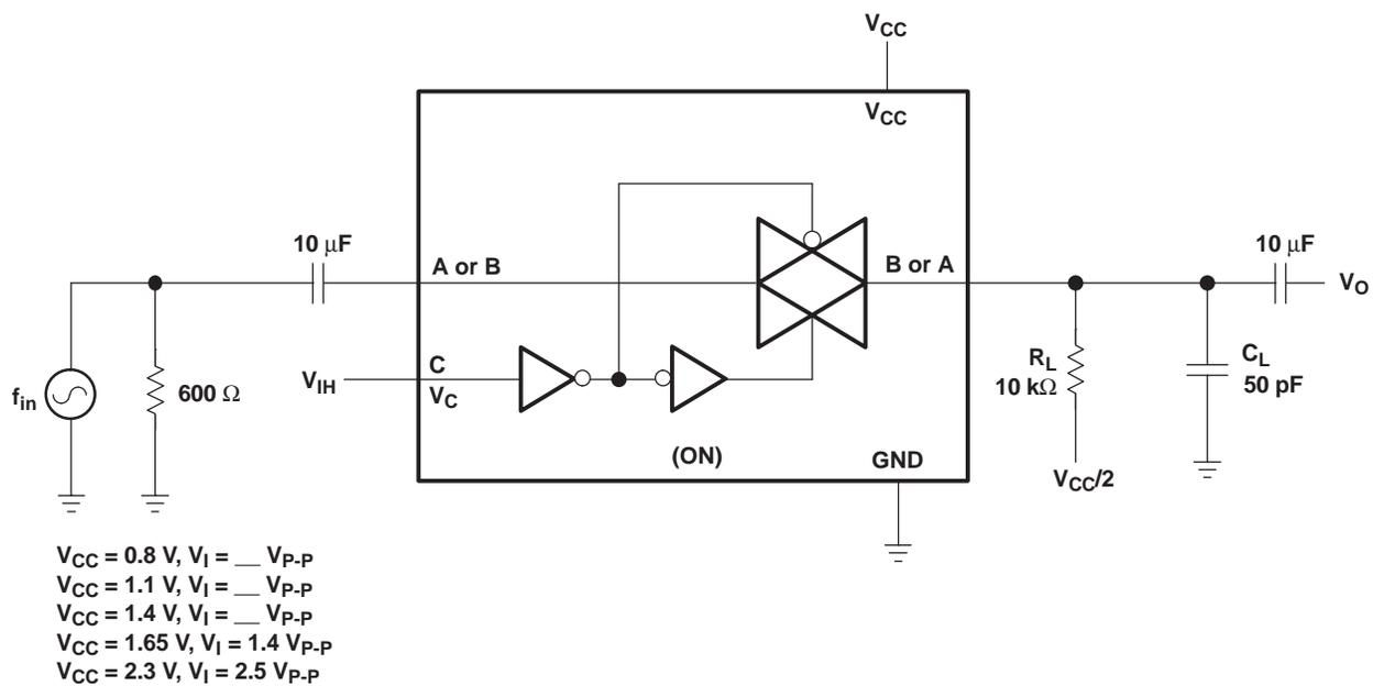
**Figure 8. Sine-Wave Distortion**
