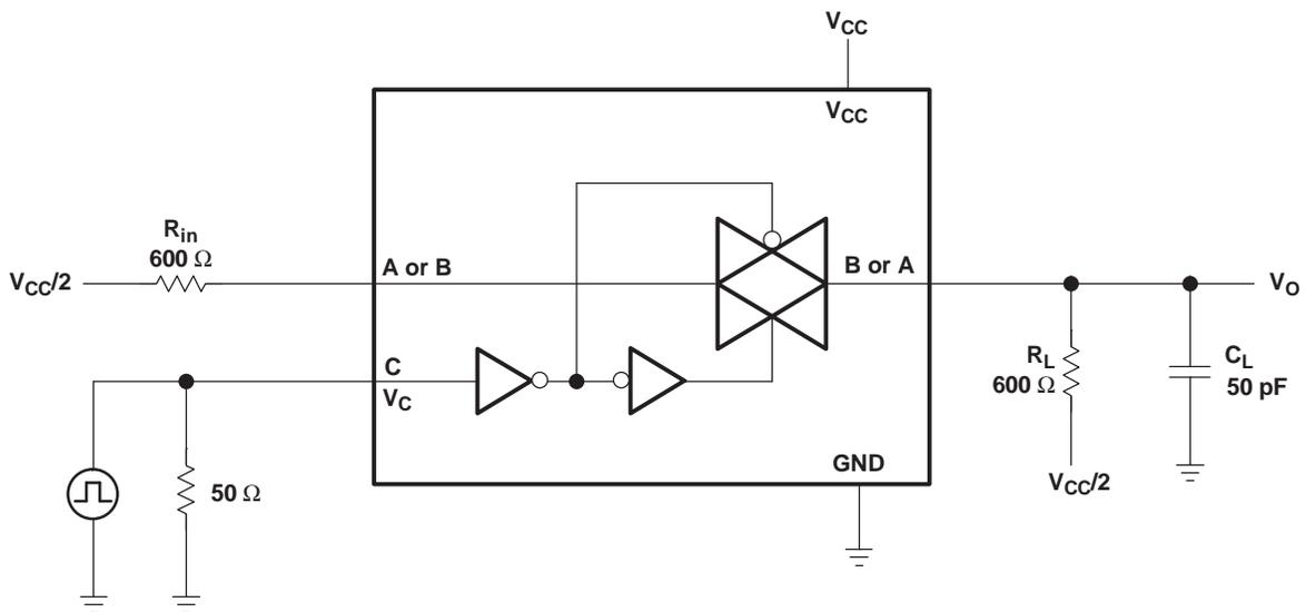
**Figure 6. Crosstalk (Control Input – Switch Output)**
