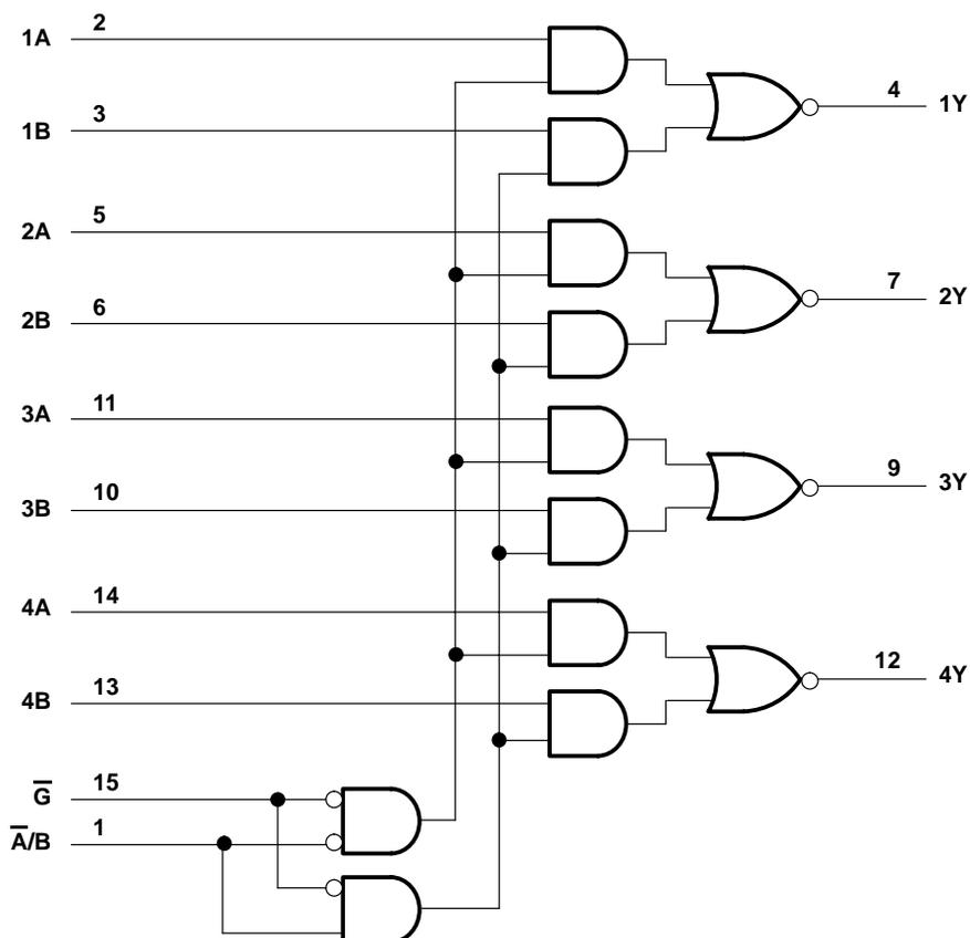
Pin numbers shown are for the D, DB, DGV, J, N, NS, PW, and W packages.
