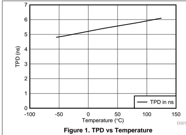
**Figure 1. TPD vs Temperature**
