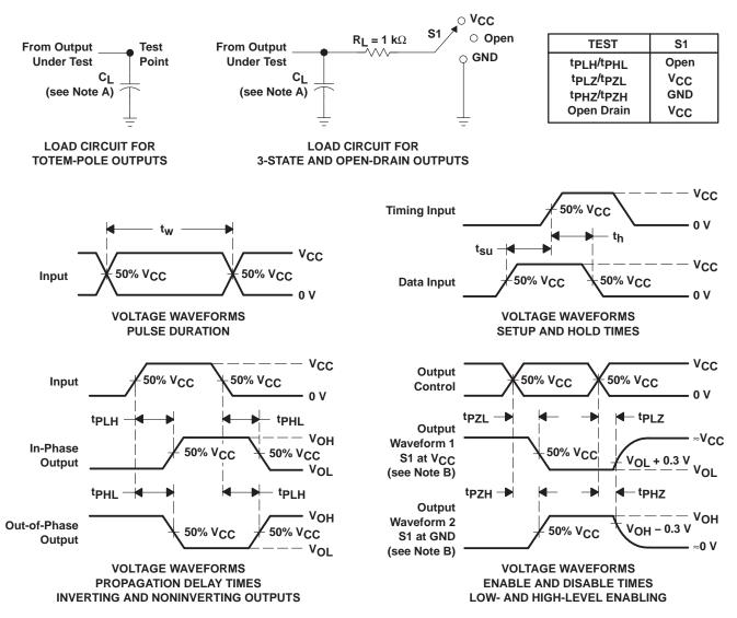
NOTES: A. C<sub>I</sub> includes probe and jig capacitance.
