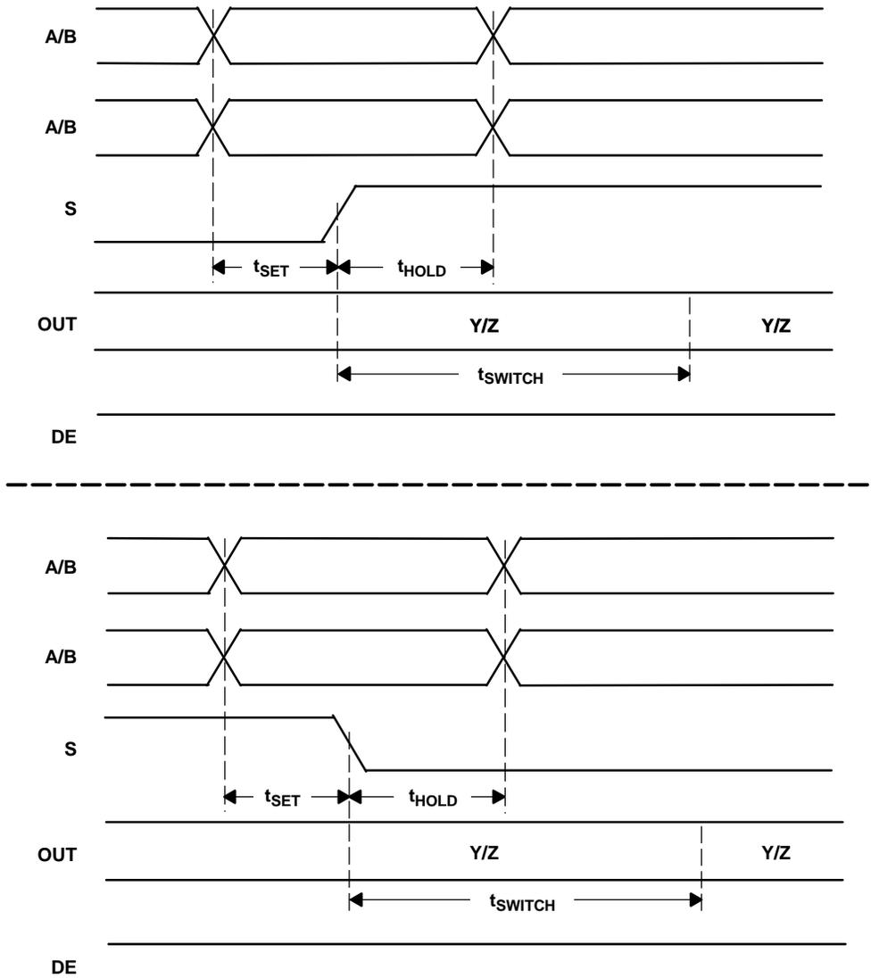
A.  $t_{SET}$  and  $t_{HOLD}$  times specify that data must be in a stable state before and after mux control switches.
