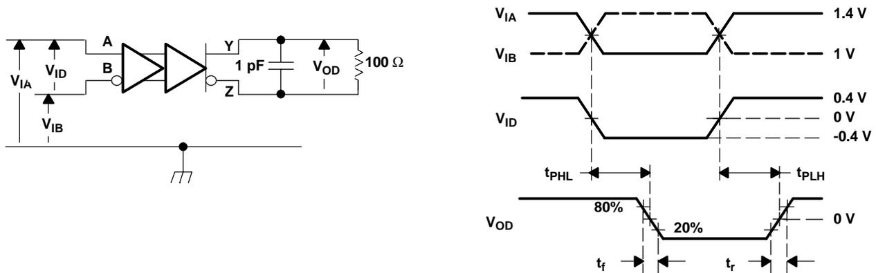
NOTE: All input pulses are supplied by a generator having the following characteristics:  $t_r$  or  $t_f \leq 0.25$  ns, pulse repetition rate (PRR) = 0.5 Mpps, pulse width =  $500 \pm 10$  ns.  $C_L$  includes instrumentation and fixture capacitance within 0,06 mm of the D.U.T.
