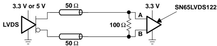
Figure 26. Low-Voltage Differential Signaling (LVDS)
