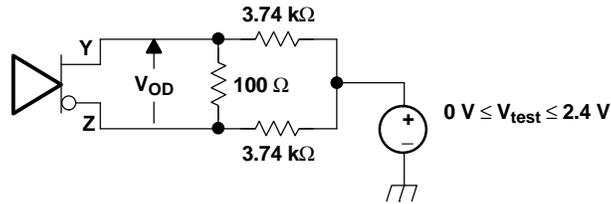
Figure 2. Differential Output Voltage ( $V_{OD}$ ) Test Circuit
