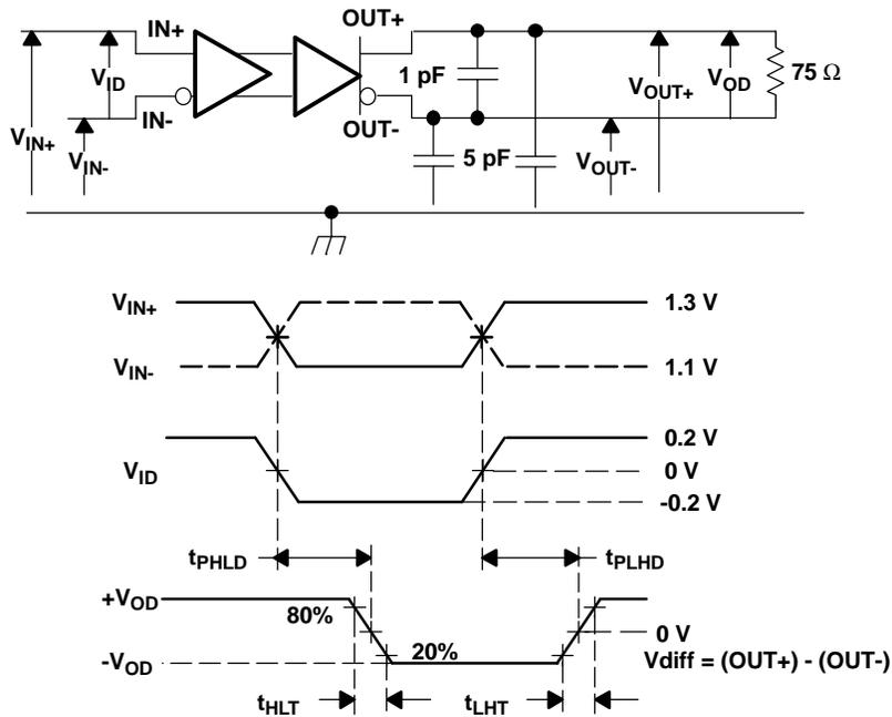
NOTE: All input pulses are supplied by a generator having the following characteristics:  $t_r$  or  $t_f \leq .25$  ns, pulse-repetition rate (PRR) = 0.5 Mpps, pulse width =  $500 \pm 10$  ns.  $C_L$  includes instrumentation and fixture capacitance within 0,06 mm of the D.U.T.
