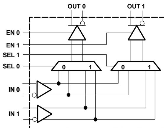
EQUIVALENT INPUT AND OUTPUT SCHEMATIC DIAGRAMS
