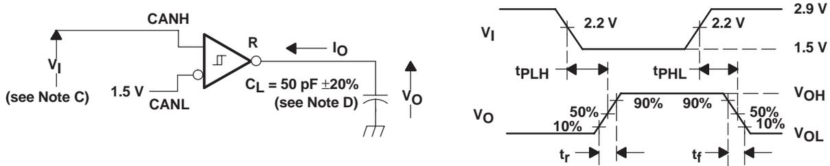
NOTES: C. The input pulse is supplied by a generator having the following characteristics: Pulse repetition rate (PRR) ≤ 125 kHz, 50% duty cycle,  $t_r \leq 6\text{ns}$ ,  $t_f \leq 6\text{ns}$ ,  $Z_O = 50\Omega$ .
