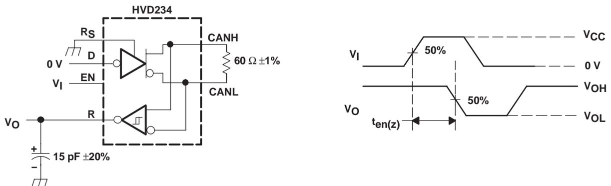
NOTE: All  $V_I$  input pulses are supplied by a generator having the following characteristics:  $t_r$  or  $t_f \leq 6$  ns, pulse repetition rate (PRR) = 50 kHz, 50% duty cycle.
