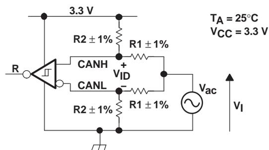
The R Output State Does Not Change During Application of the Input Waveform.
