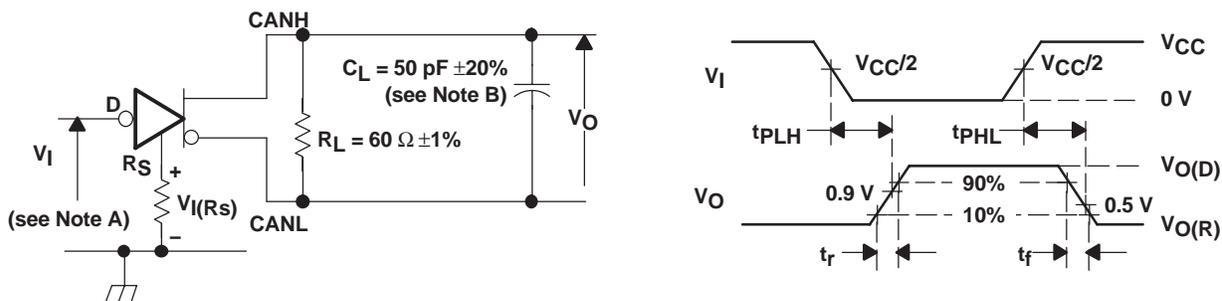
NOTES:A. The input pulse is supplied by a generator having the following characteristics: Pulse repetition rate (PRR) ≤ 125 kHz, 50% duty cycle,  $t_r \leq 6\text{ns}$ ,  $t_f \leq 6\text{ns}$ ,  $Z_0 = 50\Omega$ .
