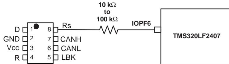
Figure 29. Slope Control/Standby Connection to a DSP
