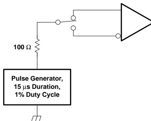
Figure 7. Overvoltage Protection
