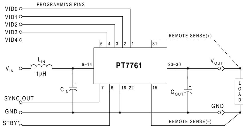
$C_{in}$  = Required 1500 $\mu$ F electrolytic
