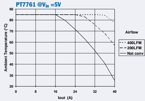
**Note A:** Characteristic data in the above graphs has been developed from actual products tested at 25°C. This data is considered typical for the ISR.
