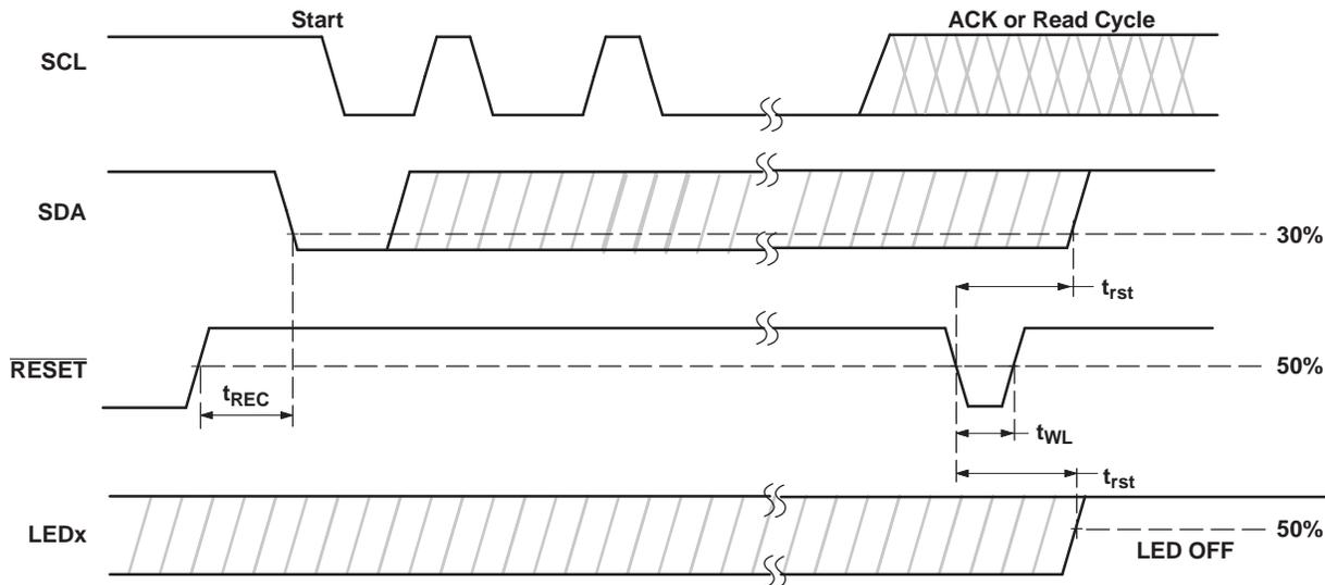
**Figure 11. Reset Timing**
