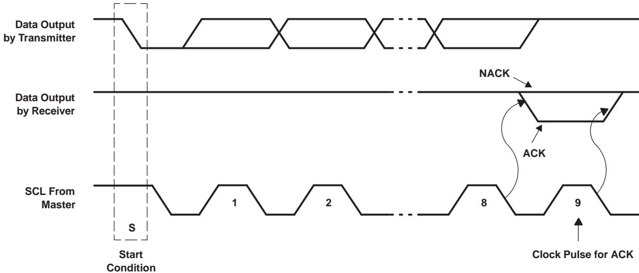
Figure 7. Acknowledgment on the I<sup>2</sup>C Bus
